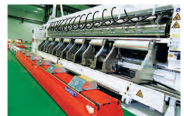
High speed slitter with web inspection camera in GMP positive pressure environment
