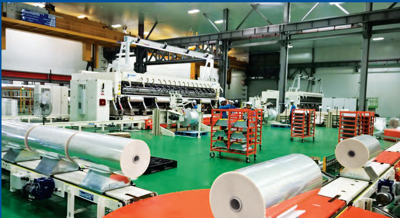
Automatic slit roll handling, conveying and packing
