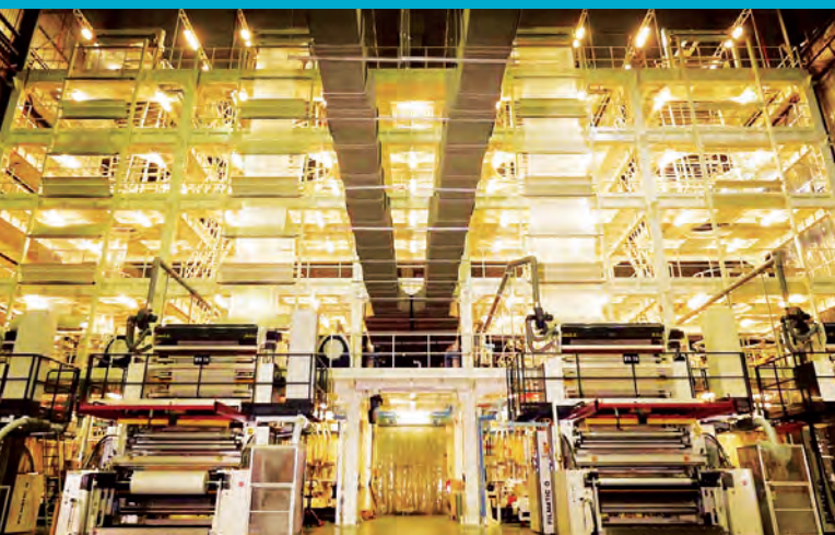
Blown film extrusion process
