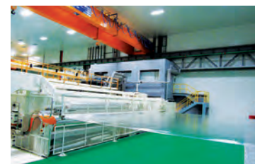
JSW's high capacity 8.8m x 525m/min BOPP film stretching plant
