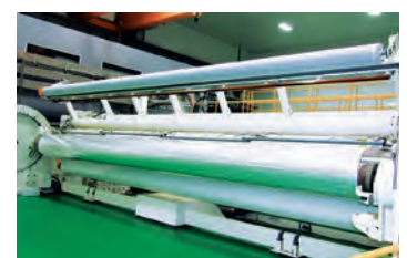
High speed slitter with web inspection camera in GMP positive pressure environment
