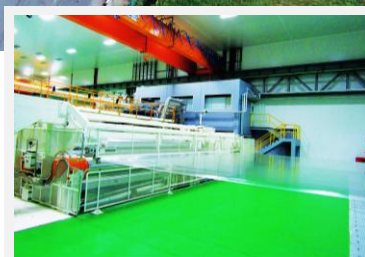
BOPP film stretching plant
